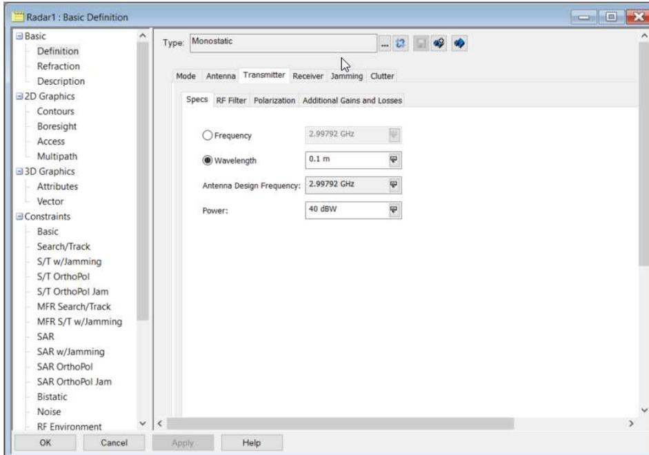
Figure 1 – Radar Transmitter Inputs
