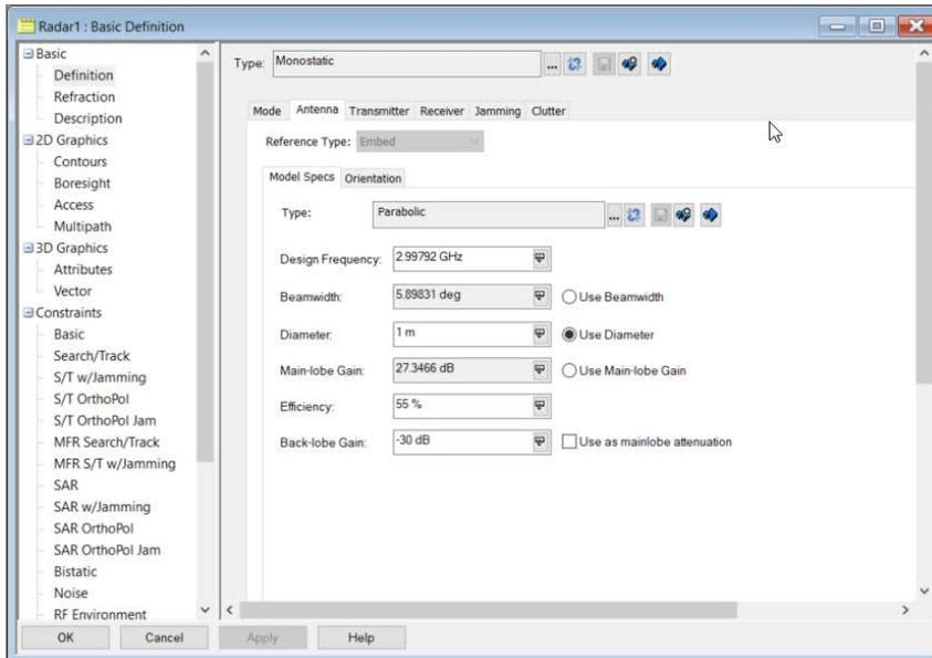
Figure 3 – Antenna Properties
