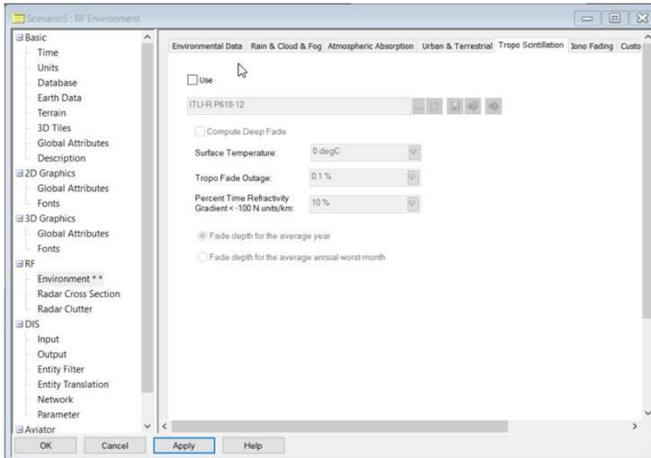
Figure 26 – RF Tropospheric Scintillation Parameters
