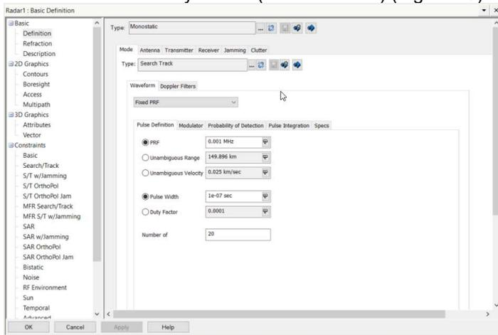
Figure 18 – Radar Pulse Definition
