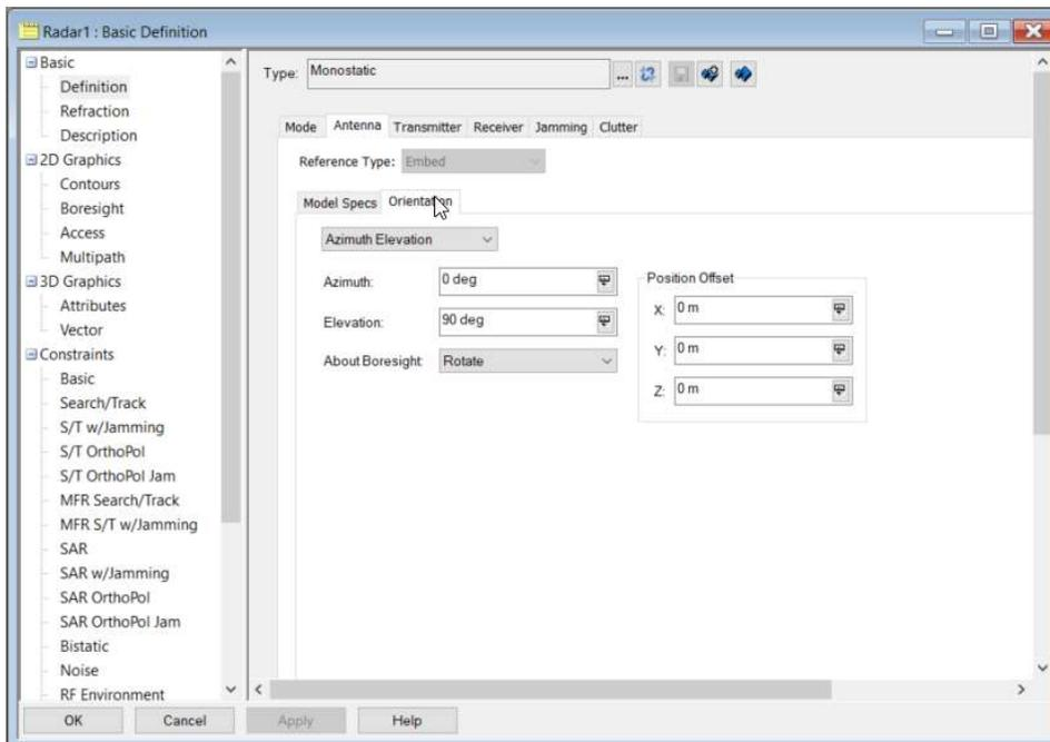
Figure 4 – Antenna Orientation Inputs
